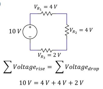
"The algebraic sum of all voltages around any closed path in a circuit is zero" (positive for a voltage rise, negative for a voltage drop.
