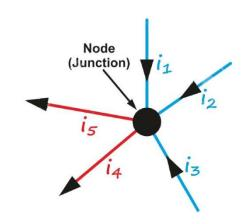
The algebraic sum of the currents entering and leaving a node is equal to zero
